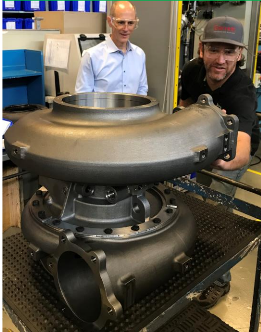
GT 80 frame-size being assembled in Torrance
