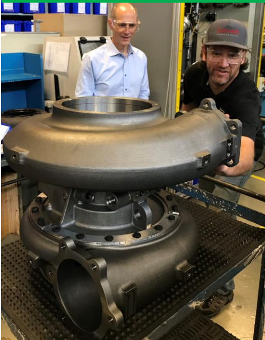
GT 80 frame-size being assembled in Torrance
