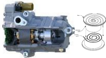
Volumetric scroll compressor 10 kRPM, oil lubricated
