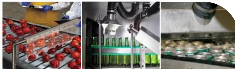
Example of “Air Knives” used in processing
