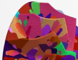
Material grain structure modeling for cast turbine wheel
